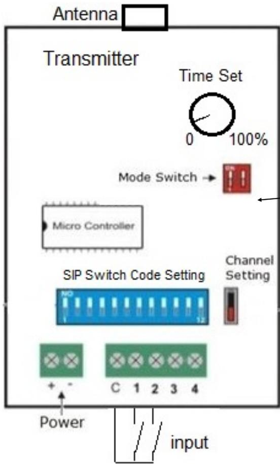
Typical wiring diagram
